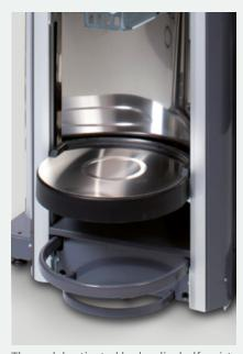
The pedal activated hydraulic shelf assists the operator in moving the can shelf when handling heavy loads.
