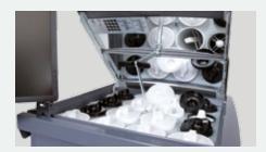
The refilling operation is made easy, both by the use of a mirror layer on the inner top lid, and by the low overall height of the machine.
