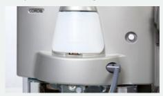
The active humidification system proves to be an ideal device for avoiding colorant drying in the nozzle area.
