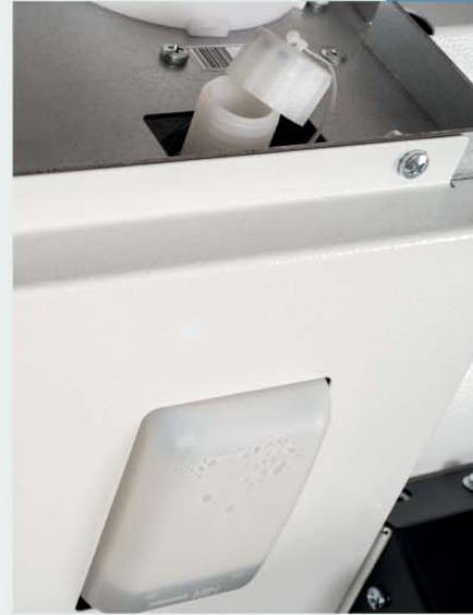
The active humidifier system works when both the cap is closed or when its open during the dispense mode for an effective protection against drying of the nozzle area.
