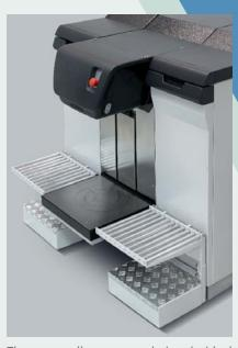
The new roll conveyor design is ideal for withstanding heavy weights, while allowing to be added after the purchase of the machine.
