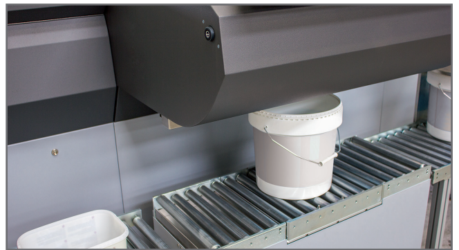
Adjustable automated roll conveyors to ensure a user-friendly and ergonomic can flow
